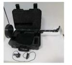
DVC # 23-91 – Laser Target Interface **Device (LTID)** – The LTID interfaces existing live-fire tank/man target mechanisms with MILES transmitters enabling MILES transmitters to knock
