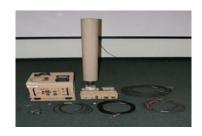
DVC # 30-35 – THOR III t Training **Device** – THOR III t system is used to train Soldiers in use of the actual THOR Il system that is used to provide protection against Remote Controlled Improvised Explosive Devices (RCIEDs)
